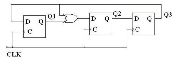
(a) Complete the next state equations (i.e.  $Q1^+$ ,  $Q2^+$ ,  $Q3^+$ ), one for each stage (flip-flop). [3 pts] (b) Assuming that  $Q_1Q_2Q_3 = 001$  at t = 0 (initialization). Determine the contents of the LFSR after the first, second, third, ..... eighth clock cycles and fill in the table given below. [3 pts]
