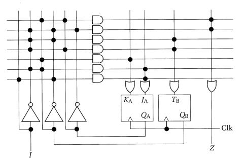
(e) Assuming the  $\overline{PR}$  is deasserted (HIGH) and the active-low clear  $\overline{CLR}$  below is connected to both flip-flops fill the timing diagram below for  $Q_A$ ,  $Q_B$  & Z.
