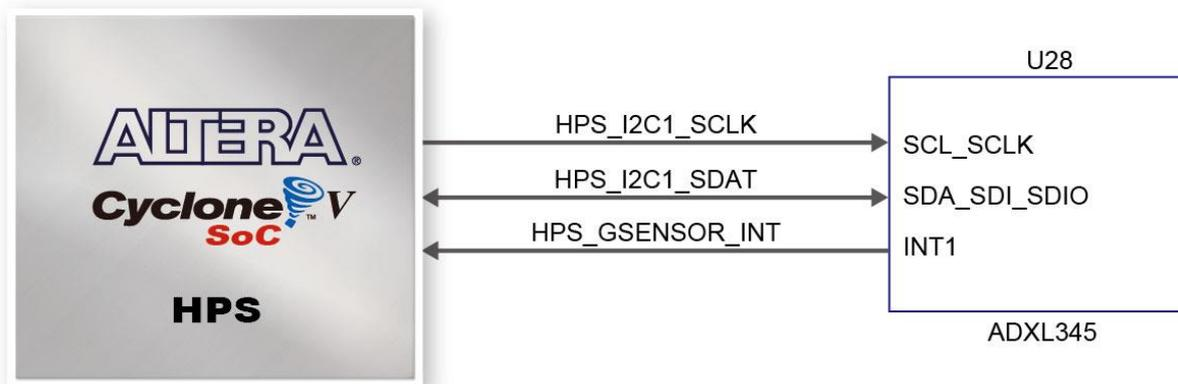
Figure 3-36 Connections between Cyclone V SoC FPGA and G-Sensor
