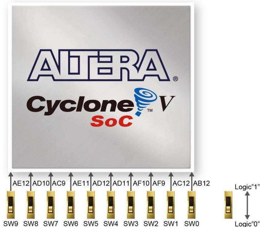
**Figure 3-16 Connections between the slide switches and the Cyclone V SoC FPGA**
