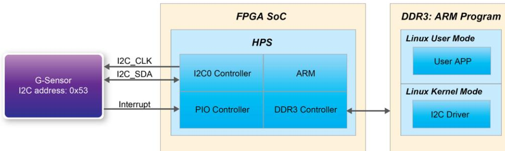
**Figure 6-6 Block diagram of the G-sensor demonstration**
