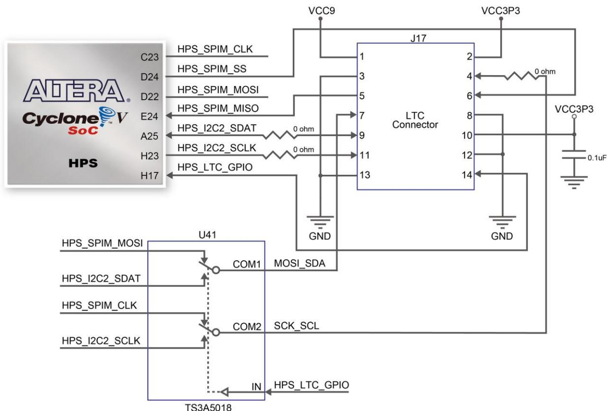
Figure 3-37 Connections between the HPS and LTC connector
