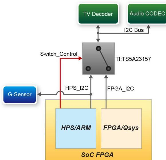
Figure 3-21 Control mechanism for the I2C multiplexer
