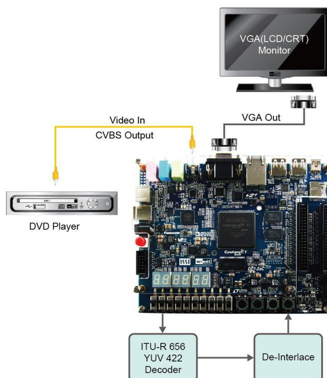
**Figure 5-10 Setup for the TV box demonstration**
