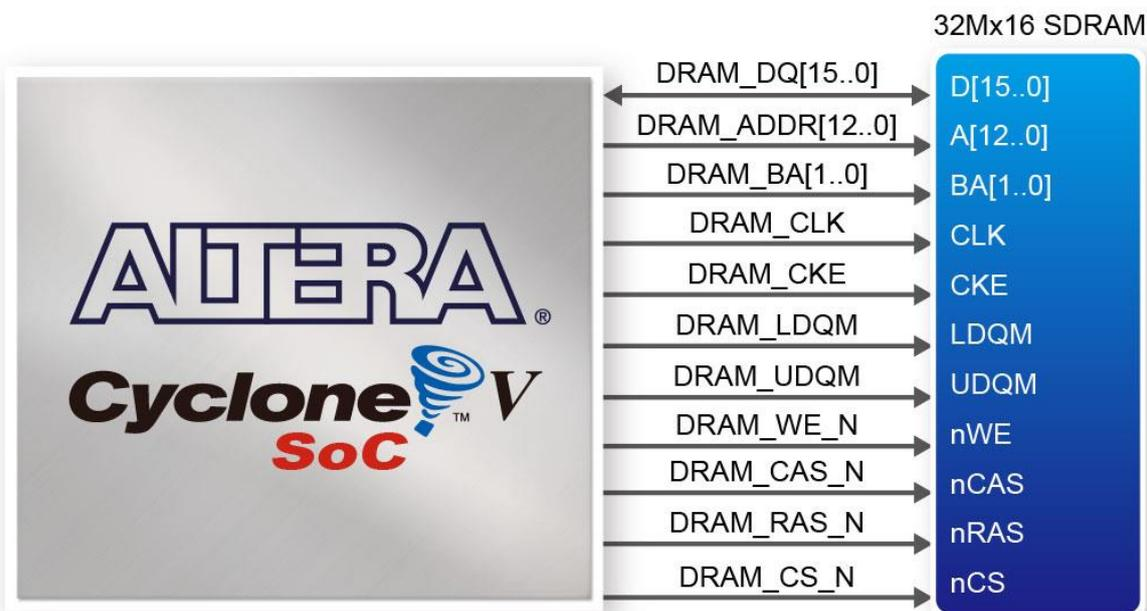
Figure 3-27 Connections between the FPGA and SDRAM
