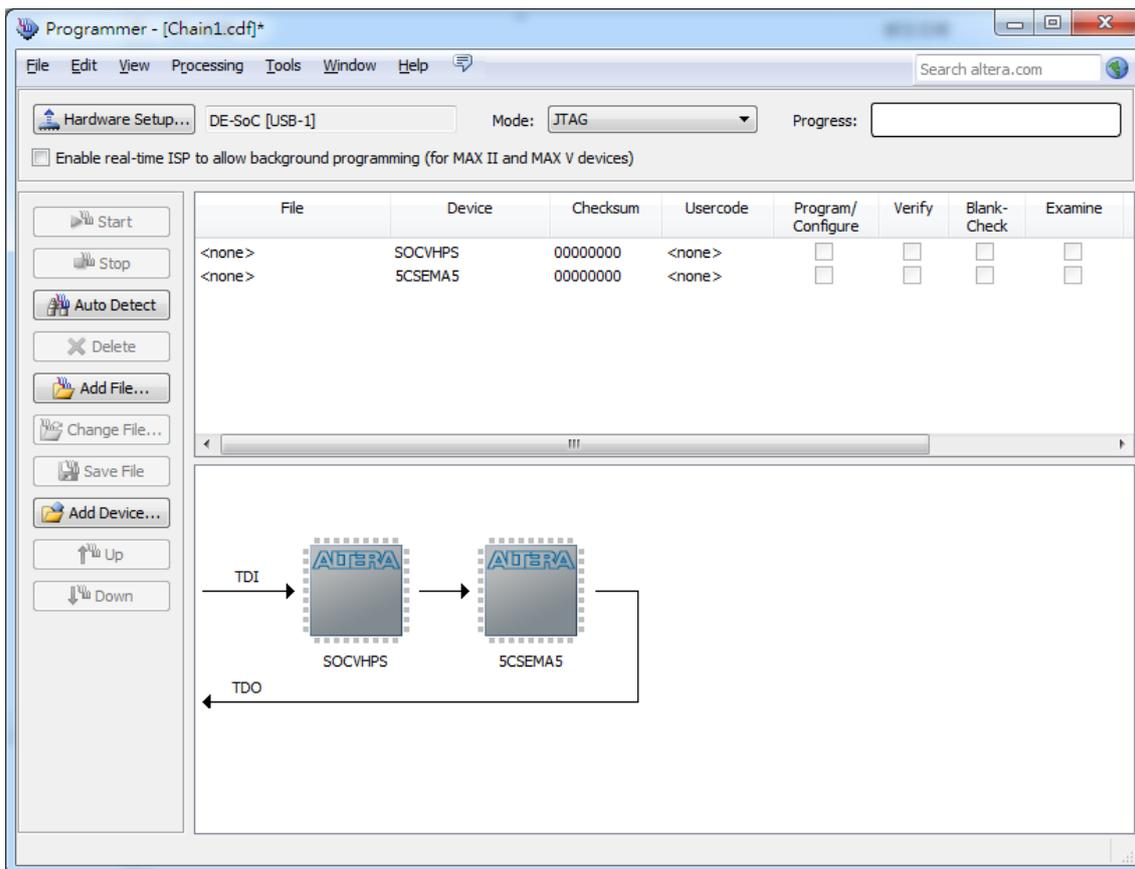
**Figure 3-5 FPGA and HPS detected in Quartus programmer**
