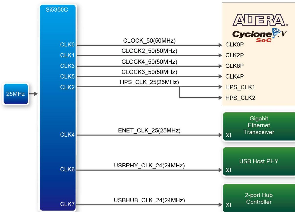
**Figure 3-13** Block diagram of the clock distribution on DE1-SoC
