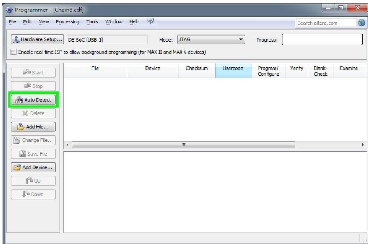
**Figure 3-3 Detect FPGA device in JTAG mode**
