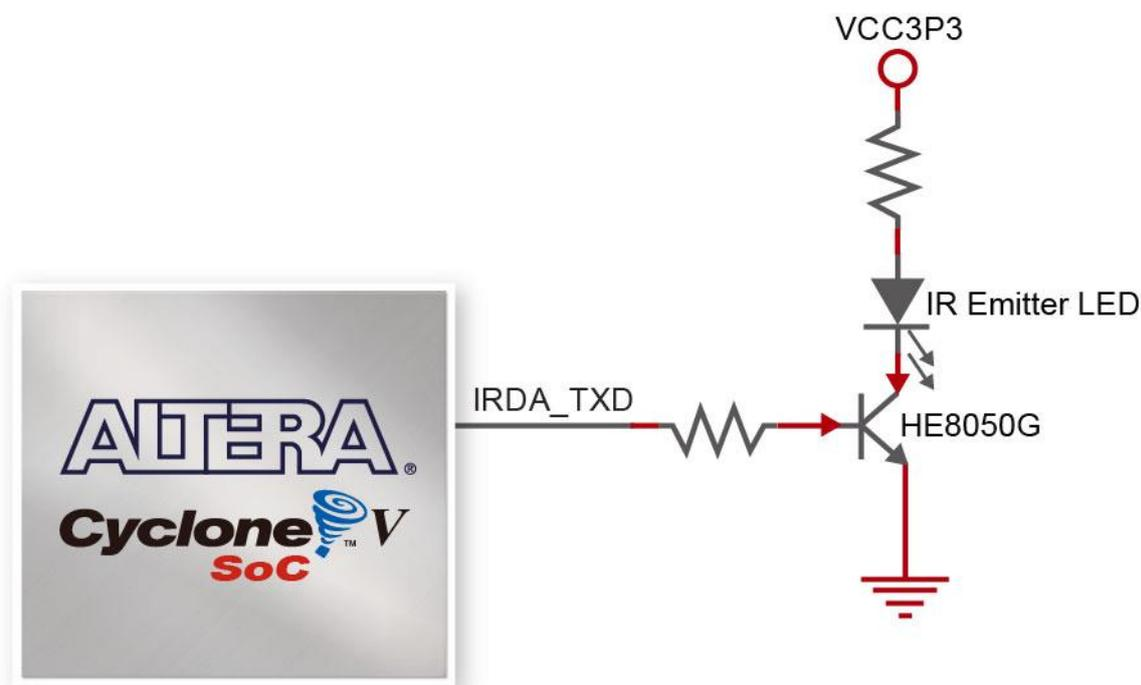
Figure 3-26 Connection between the FPGA and IR emitter LED
