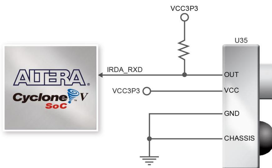
**Figure 3-25 Connection between the FPGA and IR Receiver**
