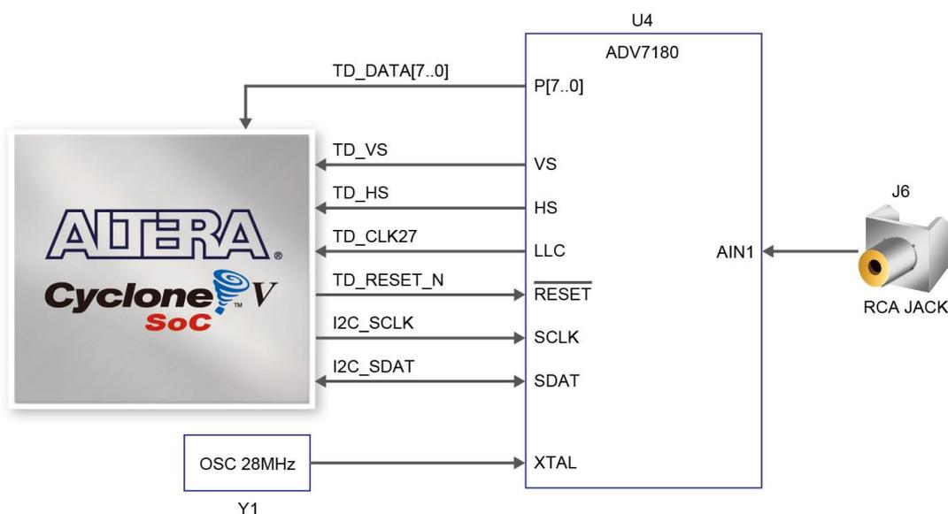
**Figure 3-24 Connections between the FPGA and TV Decoder**
