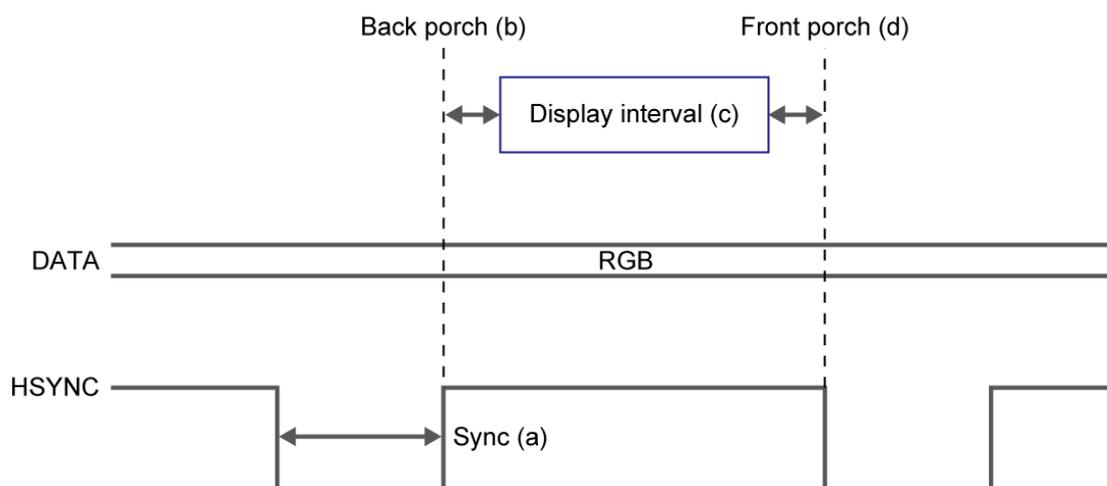
Figure 3-23 VGA horizontal timing specification
