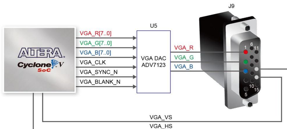
Figure 3-22 Connections between the FPGA and VGA
