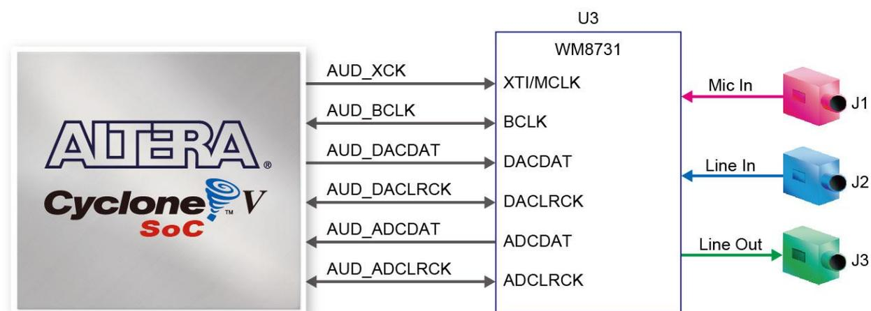
Figure 3-20 Connections between the FPGA and audio CODEC
