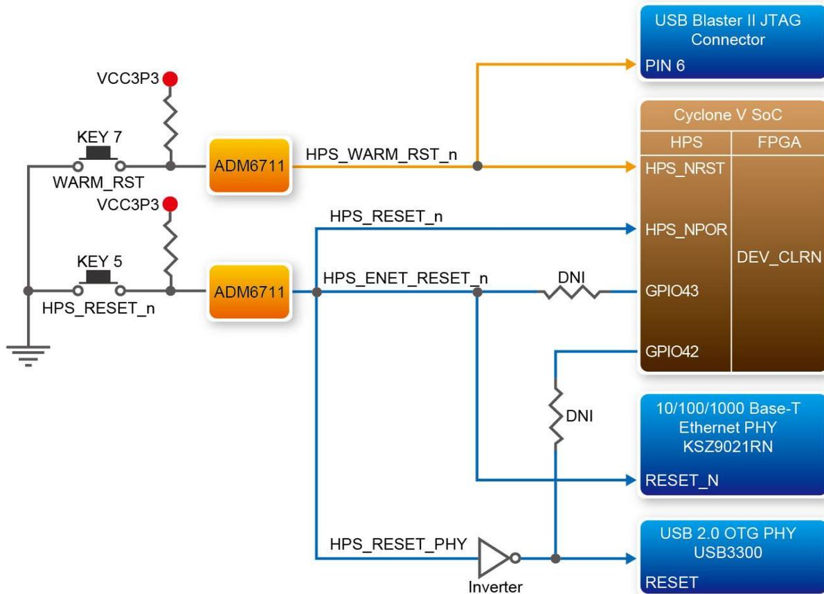
**Figure 3-12 HPS reset tree on DE1-SoC board**
