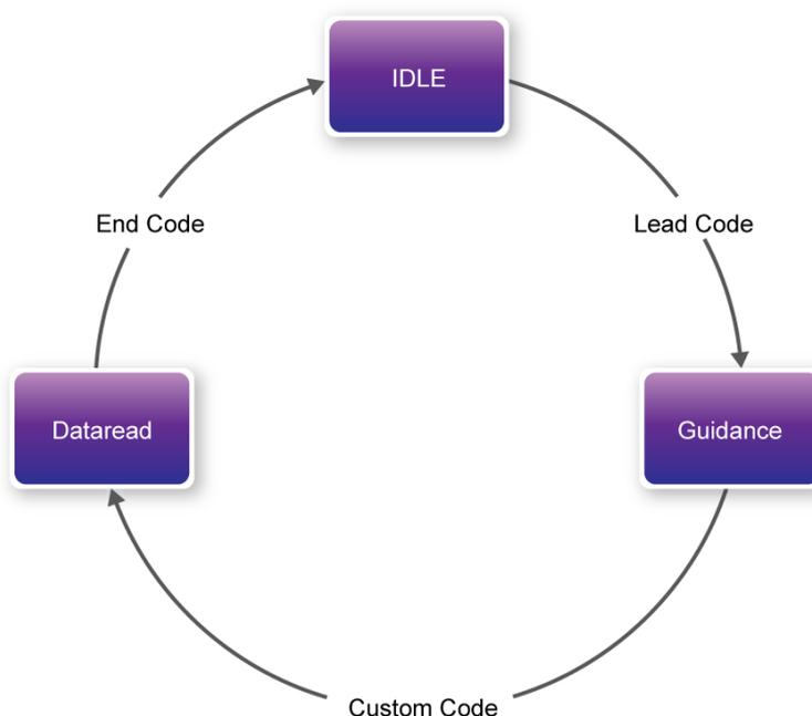
**Figure 5-18 State shift diagram of State Machine block**
