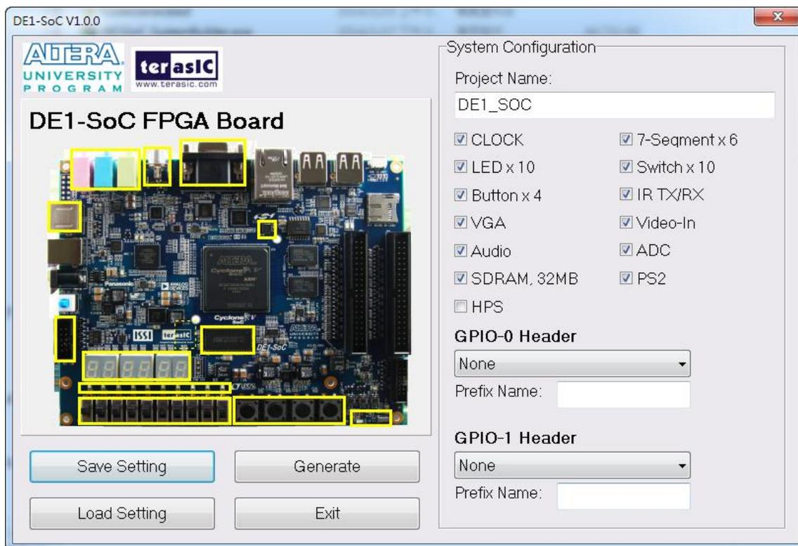
**Figure 4-2 The GUI of DE1-SoC System Builder**
