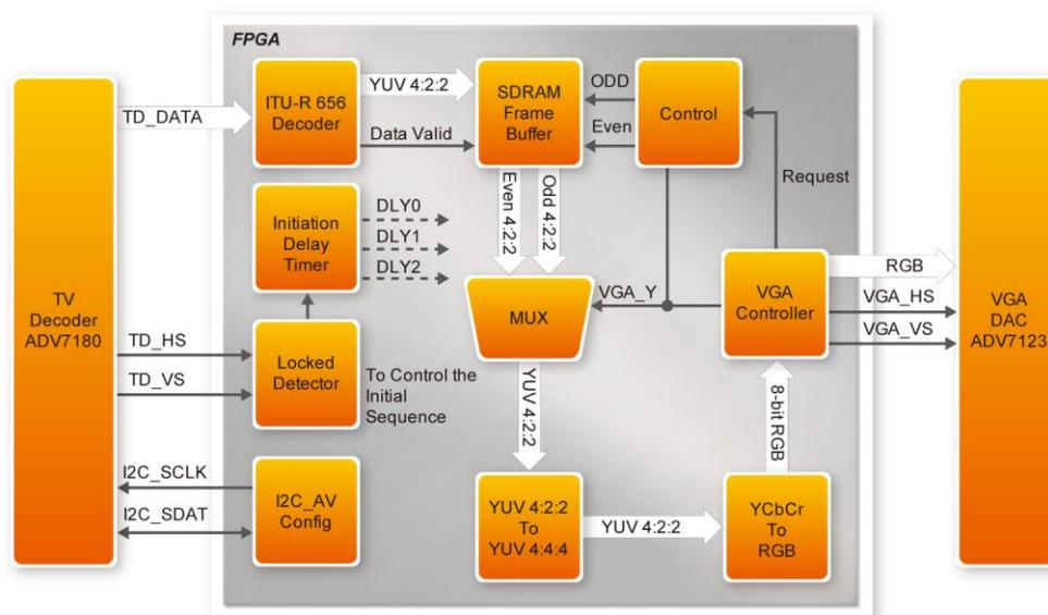
**Figure 5-9 Block diagram of the TV box demonstration**
