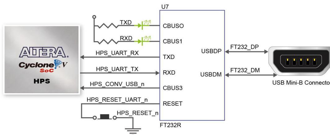
**Figure 3-33** Connections between the HPS and FT232R Chip
