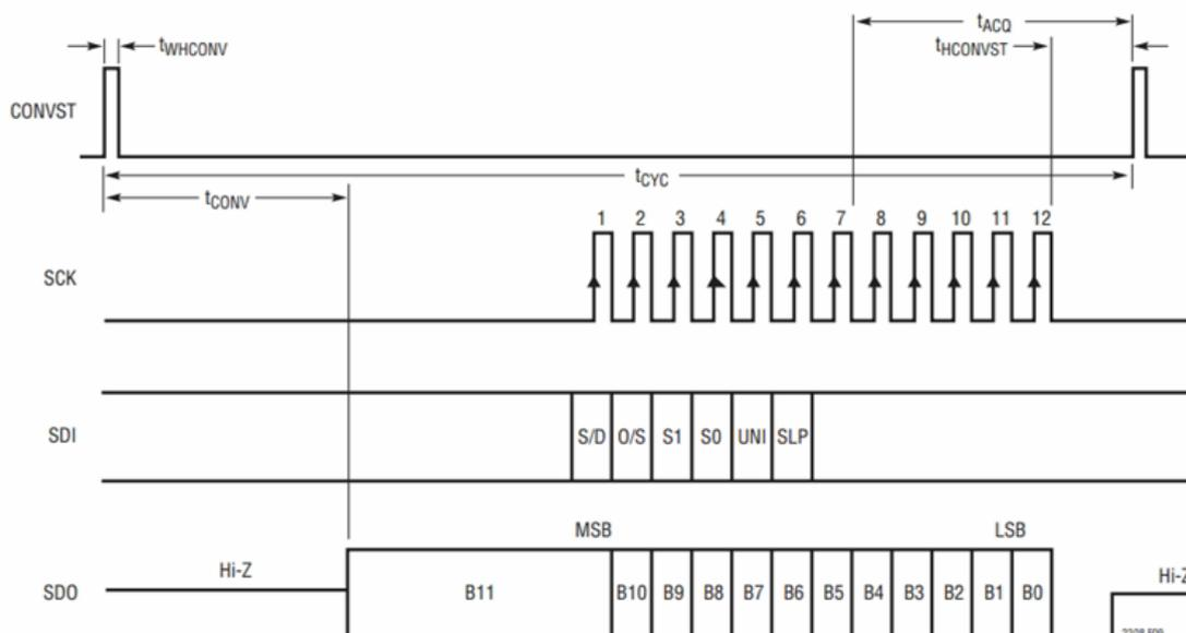
**Figure 5-21 LTC2308 Timing with a Short CONVST Pulse**
