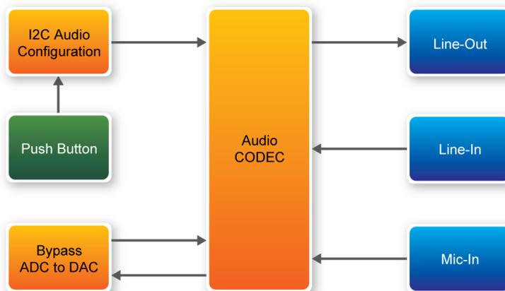
**Figure 5-4 Block diagram of the Karaoke machine demonstration**
