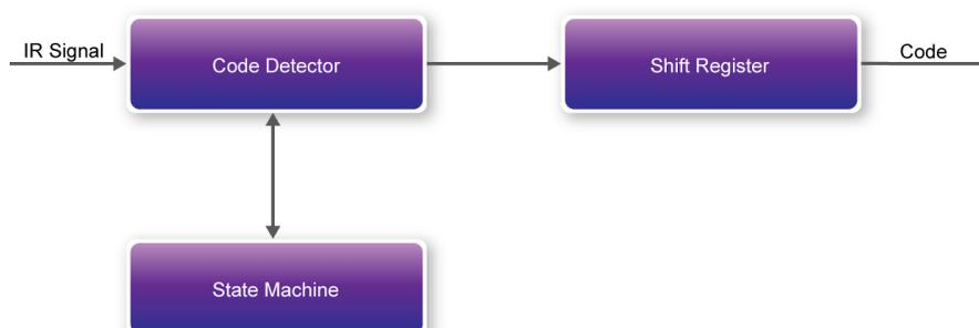
**Figure 5-17** Modules in the IR Receiver controller
