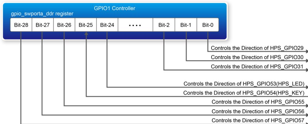
**Figure 6-5 gpio\_swporta\_ddr register in the GPIO1 controller**
