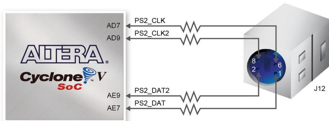
Figure 3-28 Connections between the FPGA and PS/2
