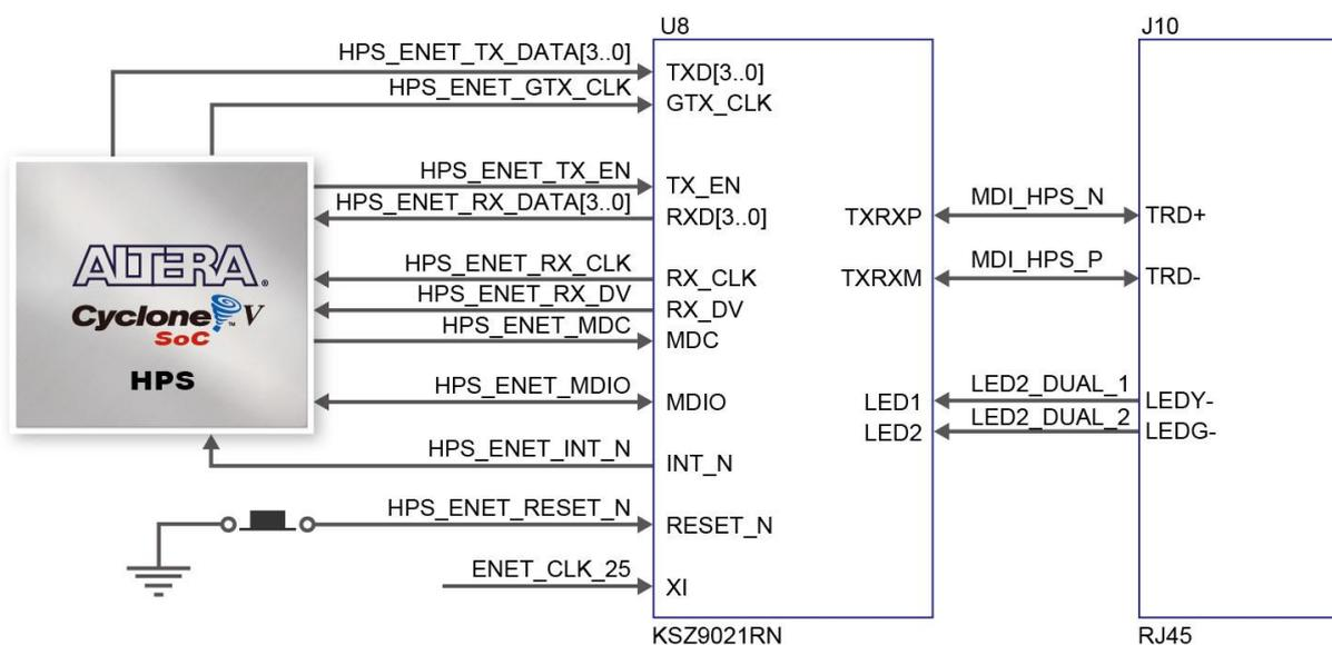
**Figure 3-32 Connections between the HPS and Gigabit Ethernet**
