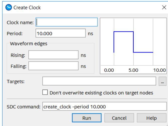
Figure 17. TimeQuest window to create a clock constraint.
