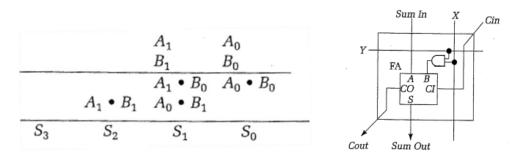
Each of the ANDed terms is called a partial product. The resulting product is formed by accumulating down the columns of partial products, propagating the carries from the rightmost columns to the left.
