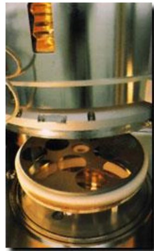
Epitaxial Reactor (Mitsubishi Materials Silicon)
