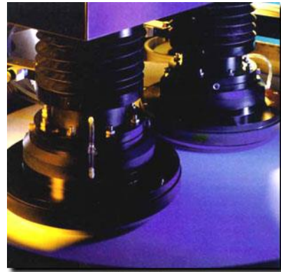
Wafer Polishing (Strasbaugh Corporation)
