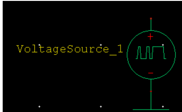
Figure 125: Grounded Voltage Source
